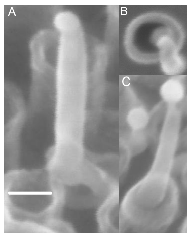
Figure 3. Scanning electron micrograph of three different CNT–ZnO hybrid structures at varying tilt angles. (A) SEM tilt angle 45°. (B) An overhead view. (C) A 30° tilt angle. The scale bar represents 50 nm.
